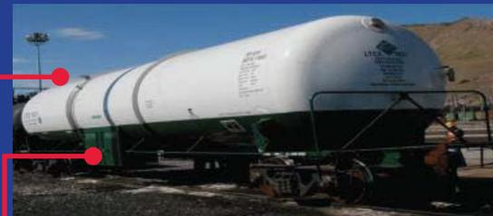
Refrigerated liquid - Argon most common - venting from pipes up the side of the car is normal operation.
